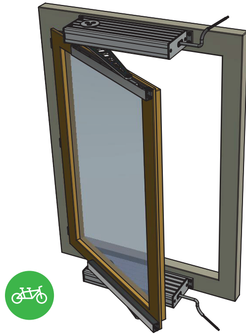
Figure 8: Installation sequence TANDEM installation
